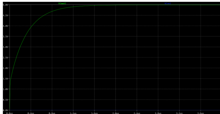
Figure 10: Simulation result displaying amplification of signal to 5V
